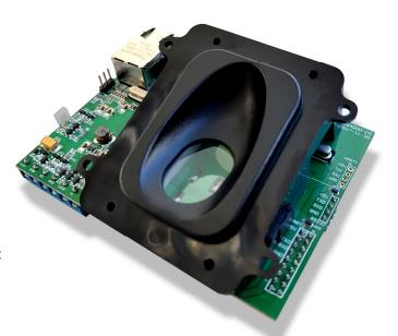
FS84C has 1 output channel (for external relay control) and 2 input channels(for door sensor and switch). So it can be used as a fingerprint access control device.
